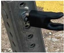
Figure 6 Locator tried to improving grounding by connecting to a larger and deeper grounding connection - a stop sign.
