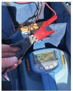
Figure 4 Locator confirms connection leads are in working order by clipping them together and confirming current flow.
