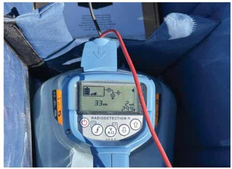
Figure 2 Signal transmitter shows 29.9 volts of electrical pressure with only 2 mA of current flow achieved.
