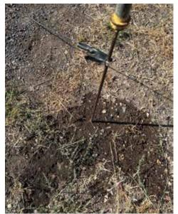
Figure 5 Locator tried improving grounding conditions by adding water to the ground stake
